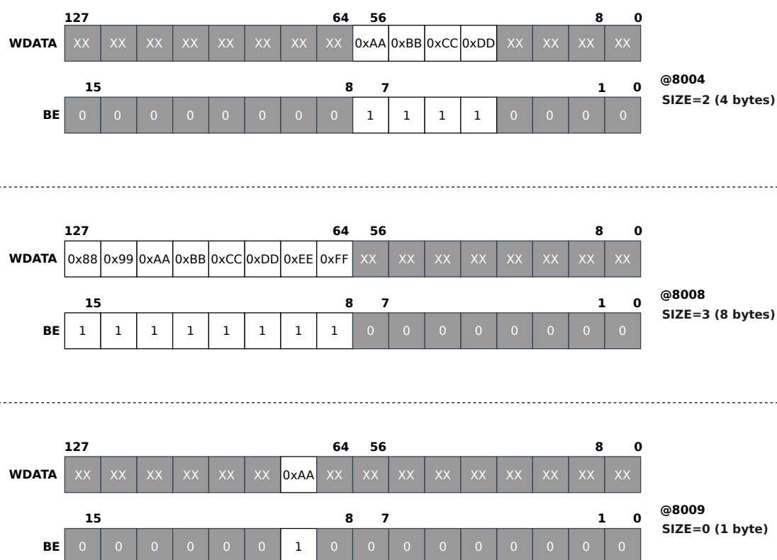
Figure 2.2: Address, Data and Byte Enable Alignment in Requests
