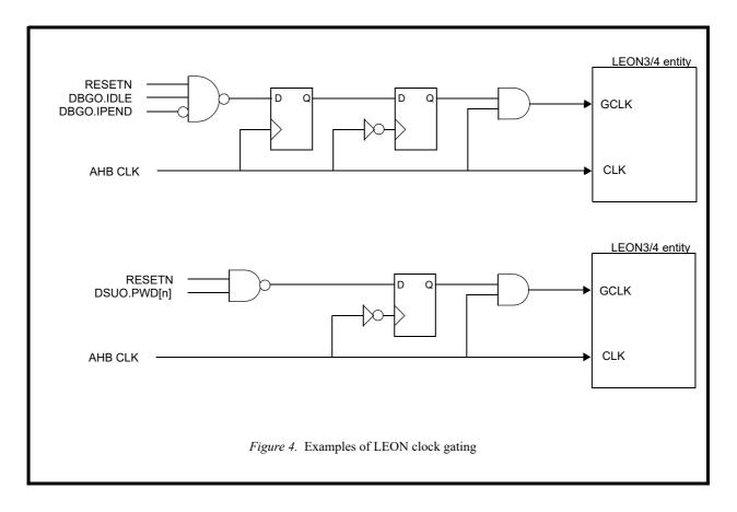
The processor should exit the power-down state when an interrupt become pending. The signal DBGO.ipend will then go high when this happen, and should be used to re-enable the clock.
