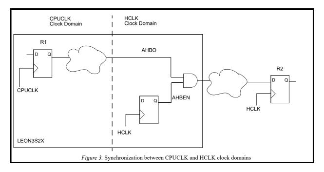
The AND gates in figures 2 and 3 are 2-input clock AND gates. Synthesis tool should not optimize these AND gates. Sample DC-script puts 'don't-touch' attribute on these cells to prevent optimization.
