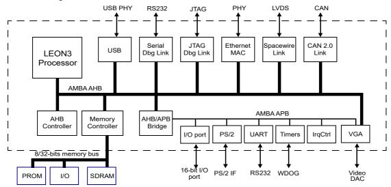
Building the system around one AHB bus has advantages in that it simplifies system design.
