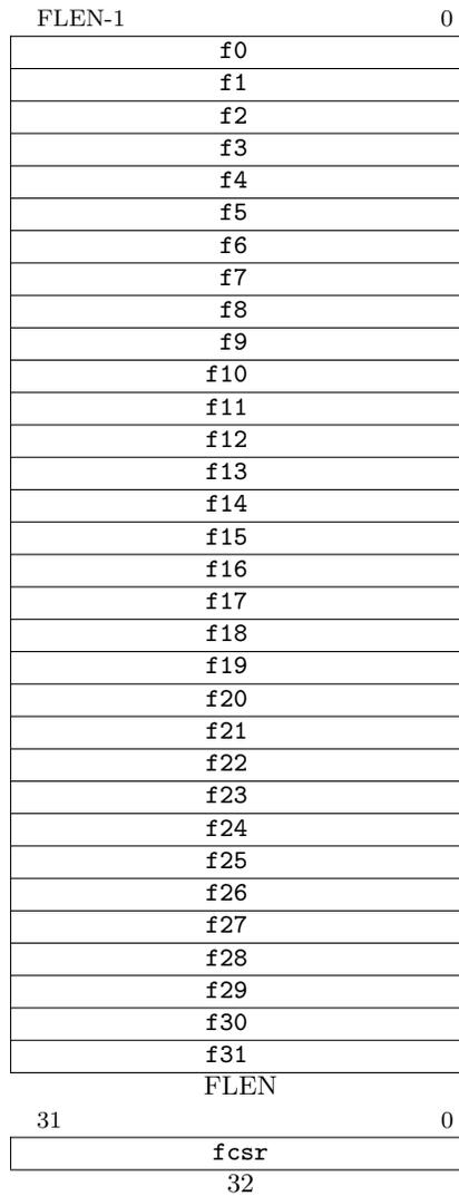
Figure 11.1: RISC-V standard F extension single-precision floating-point state.
