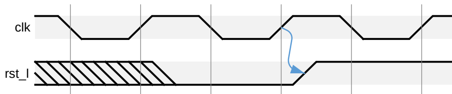
Figure 14-10 Conceptual Clock and Reset Timing Relationship
